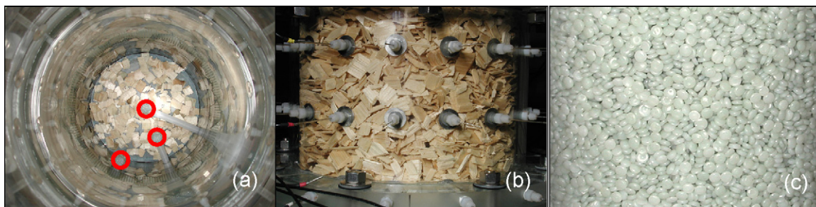
Fig. 2. Photographs of (a) the interior of the digester showing the locations of the injection tubes used for isokinetic tracer introduction. The feed tubes (highlighted in the picture) were positioned 13.5 cm above the digester base at r/R values of 0, 0.5 and 0.91; (b) side view of packed column of wood chips (for reference, the inside diameter of the vessel is 28 cm); and (c) side view of packed column of HDPE pellets (diameter of 4.4 mm).
